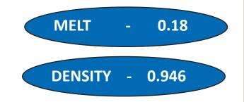
*MMF-1444* is a high molecular weight, hexene copolymer tailored for blown film applications that require toughness and durability, good processability and good blending characteristics with HDPE and HMW resins. *MMF-1444* complies with FDA regulation 21CFR 177.1520 (c) 3.2(a) and most international regulations concerning the use of Polyethylene in contact with food.
