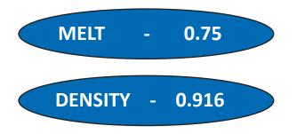
**LLHF-116XF** is a certified prime, Super-Hexene copolymer developed for blown film with outstanding impact strength and toughness. **LLHF-116XF** complies with FDA regulation 21CFR 177.1520, covering safe use of polyofin articles intended for direct food contact, and with most international regulations concerning the use of Polyethylene in contact with food articles.
